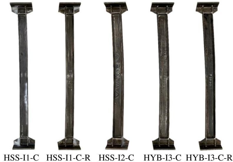
Fig. 12. Failure modes of tested welded I-section columns
