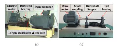
Fig. 3. Rolling bearing test platform. (a) CWRU test platform. (b) PT100 test platform.
