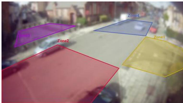
FIGURE 21: The turning zones at the HRS
