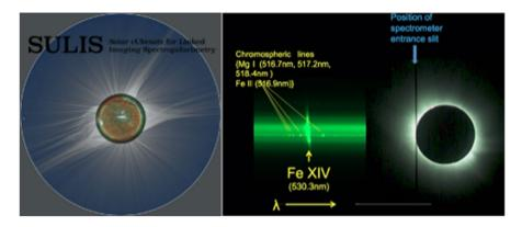
**Fig. 4** *Left:* The spectro-polarimeter (occulting CubeSat) will observe the solar disc and inner atmosphere. The coronagraph (coronagraph CubeSat) will observe extended coronal structures and CMEs. *Right:* Example of the spectrometer eclipse measurements. The slitjaw image on the right shows the slit position, the high-resolution spectra are on the left
