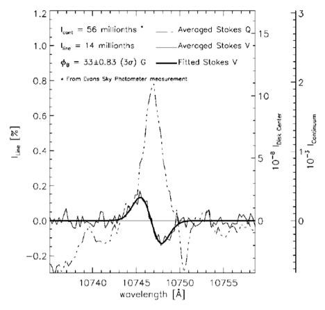
**Fig. 2** Stokes *Q* and *V* profiles averaged over the entire FOV for the observations reported in [19]. The magnetic antisymmetric profile of the Stokes *V* spectrum is clearly shown. The calibration to disc-centre intensity was obtained from a sky brightness measurement using the National Solar Observatory (NSO) Evans Sky Photometer
