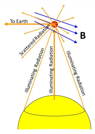
**Fig. 1** Conceptual description of the saturated Hanle Effect, whereby the yellow sphere represents the Sun, the orange lines represent the photospheric radiation emanating from the Sun surface, the blue lines are the magnetic field lines in the corona and the red circle is an ionised atom scattering the photospheric radiation
