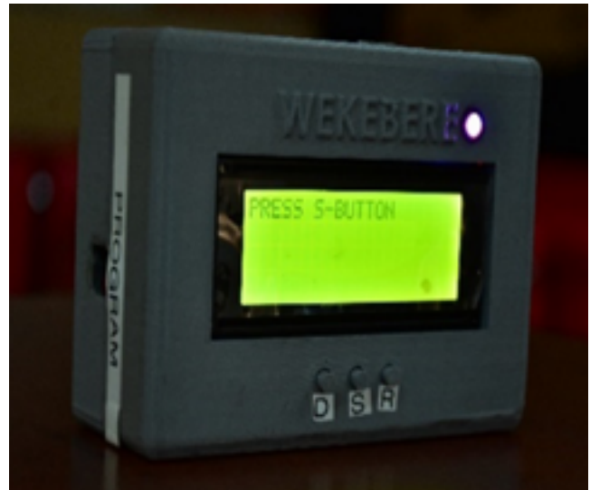
Figure 1: The Wekebere foetal heart rate device Photo credit: Stephen Tashobya, CEO Wekebere Ltd
