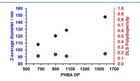
**Figure 6.** Variation in *z*-average diameter and polydispersity determined *via* DLS studies of a series of kinetically-trapped PGMA<sub>300</sub>-PHBA<sub>x</sub> spheres prepared at 30 °C when targeting a PHBA DP (*x*) ranging from 660 to 1580 at 20% w/w solids. [N.B. Targeting even higher PHBA DPs merely resulted in substantially incomplete HBA conversions (<90%) under the same conditions].
