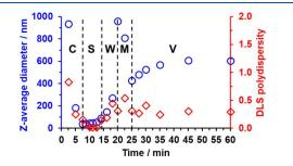
**Figure 2.** Evolution in *z*-average diameter and polydispersity determined by DLS studies during the synthesis of  $PGMA_{100}$ -PHBA<sub>650</sub> diblock copolymer nano-objects *via* RAFT aqueous dispersion polymerization of HBA using a KPS/AsAc redox initiator at 30 °C when targeting 20% w/w solids. Aliquots were extracted periodically over 60 min. [N.B. C, S, W, M, and V denote chains, spheres, worms, a mixed phase comprising worms and vesicles, and vesicles, respectively].
