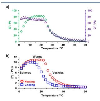
**Figure 7.** Temperature-dependent rheology studies of a 10% w/w aqueous dispersion of linear PGMA<sub>100</sub>-PHBA<sub>325</sub> nano-objects recorded at an applied strain of 1.0% and an angular frequency of 1.0 rad s<sup>-1</sup>: (a) storage (G'; green diamonds) and loss (G''; purple triangles) moduli; (b) complex viscosity (heating ramp = red data; cooling ramp = blue data). For each measurement, 2.0 min was allowed for thermal equilibration.
