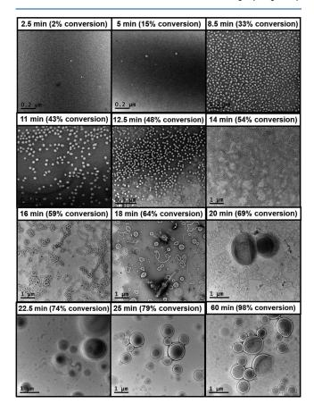
Figure 3. Representative TEM images obtained for aliquots extracted over 60 min during the synthesis of  $PGMA_{100}$ -PHBA<sub>650</sub> vesicles *via* RAFT aqueous dispersion polymerization of HBA, illustrating the progressive evolution in the copolymer morphology from spheres to worms to vesicles. In each case, the nano-object morphology was covalently stabilized at 0.1% w/w solids using excess GA cross-linker at 30 °C (to mimic the PISA synthesis conditions).
