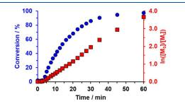
Figure 1. Conversion vs time curve (blue circles) and the corresponding semilogarithmic plot (red squares) obtained for the RAFT aqueous dispersion polymerization of HBA using a KPS/AsAc redox initiator at 30 °C when targeting  $PGMA_{100}$ -PHBA<sub>650</sub> diblock copolymer nano-objects at 20% w/w solids at a  $[PGMA_{100}]/[KPS]$  molar ratio of 10.
