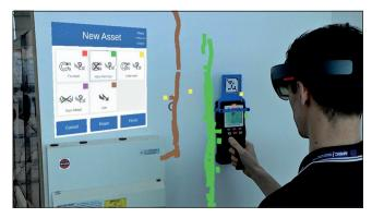
Figure 5. An example of data capture with a Microsoft Hololens headset and a Bosch D-Tect handheld wall scanner
