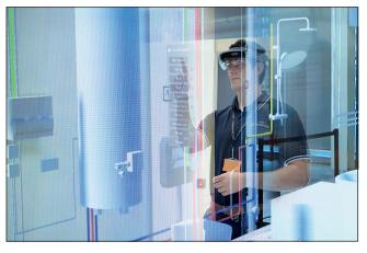
Figure 2. Microsoft Hololens headsets allow users to see a virtual overlay on a physical asset
