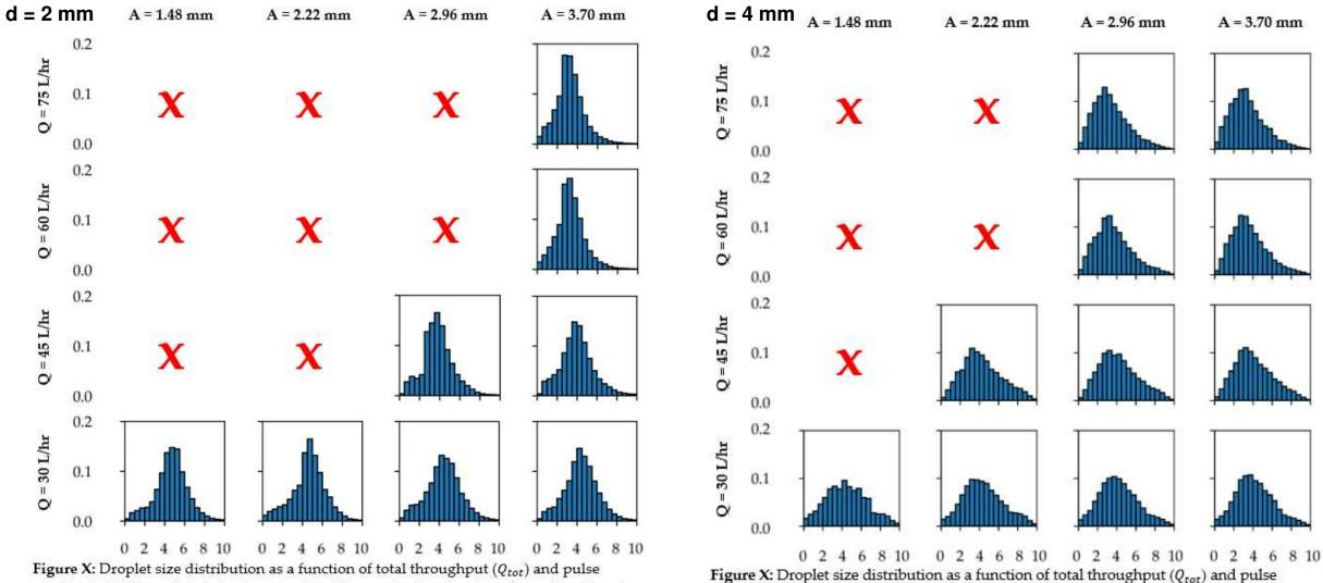
amplitude (A) for a plate hole diameter (d) of 2 mm. A red x donates column flooding at the particular operating conditions.
