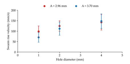
**Figure X:** Droplet swarm averaged rise velocities for a total throughput ( $Q_{tot}$ ) of 30 L/hr for pulse amplitudes (A) of 2.96 mm and 3.70 mm.
