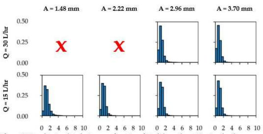
**Figure X:** Droplet size distribution as a function of total throughput ( $Q_{tot}$ ) and pulse amplitude (A) for a plate hole diameter (d) of 1 mm. A red x donates column flooding at the particular operating conditions.
