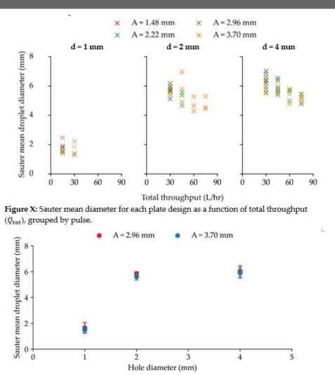
**Figure X**: Sauter mean droplet diameter for a total throughput ( $Q_{tot}$ ) of 30 L/hr for pulse amplitudes (*A*) of 2.96 mm and 3.70 mm.
