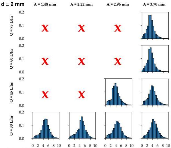
**Figure X:** Droplet size distribution as a function of total throughput  $(Q_{tot})$  and pulse amplitude (*A*) for a plate hole diameter (*d*) of 2 mm. A red x donates column flooding at the particular operating conditions.
