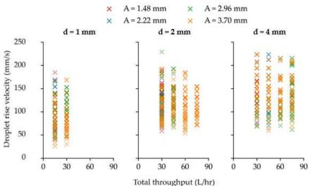
**Figure X:** Droplet rise velocities for each plate design as a function of total throughput  $(Q_{tot})$ , grouped by pulse.
