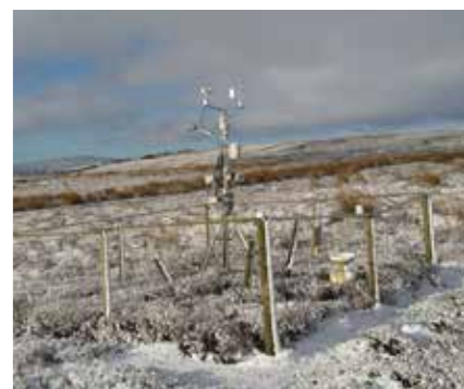
Automated weather (climate) station
