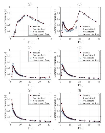
Figure 9 – Damping efficiency comparisons for varying vibration amplitudes at (a) 20 Hz, (b) 40 Hz, (c)
