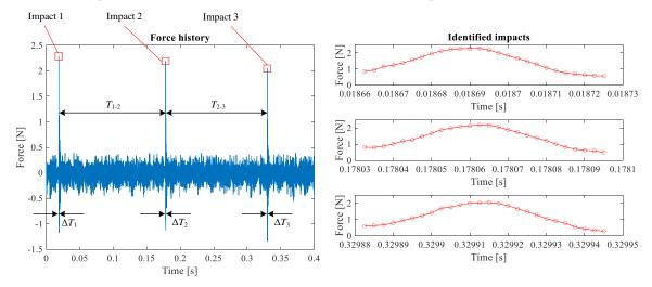
Figure 5 – A sample drop test measurement.
