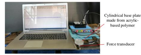
Figure 4 – Simple drop test rig.
