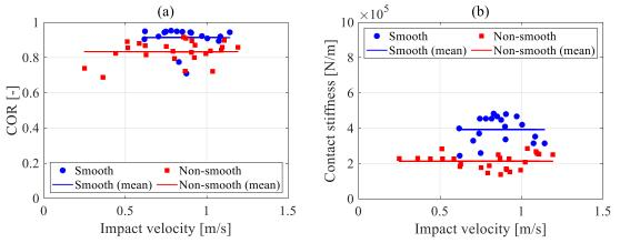
Figure 7 – Measured collisional properties: (a) COR and (b) contact stiffness.
