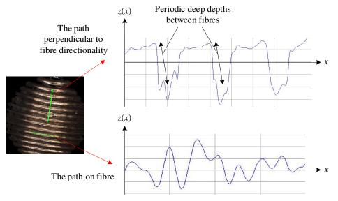
Figure 3 – Demonstration of different path directions on the non-smooth particle.
