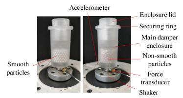
Figure 8 – Granular energy dissipation measurement rig with smooth and non-smooth particles.
