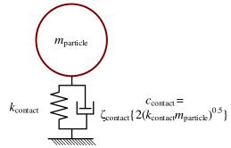
Figure 6 – Single-degree-of-freedom model of an individual impact.
