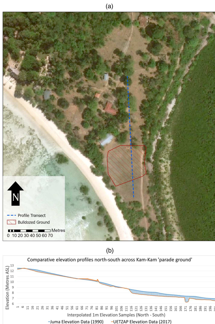
FIGURE 7 (a) MAXAR satellite image (2004) of Unguja Ukuu showing Kam-Kam and bulldozed area of parade ground, and (b) comparative elevation profiles of area of parade ground before and after bulldozing derived from Juma (2004) and UETZAP GPS surveys. UETZA, Urban Transitions and Ecology on the Zanzibar Archipelago Project; GPS, Global Positioning System. [Colour figure can be viewed at wileyonlinelibrary.com ] wileyonlinelibrary.com
