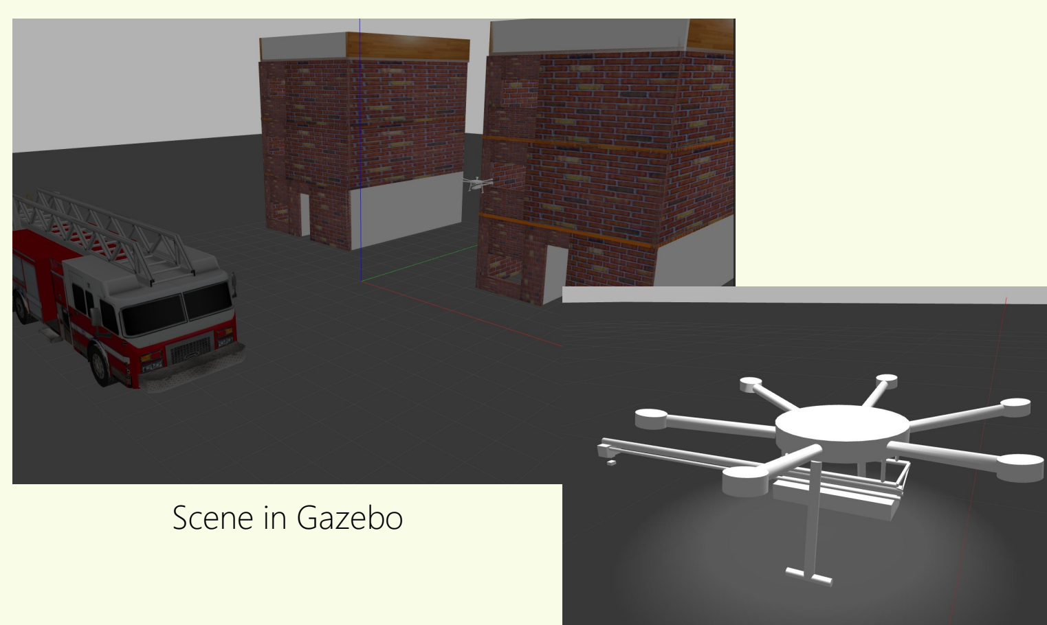
UAV model rendered in Gazebo after importing generated SDF
