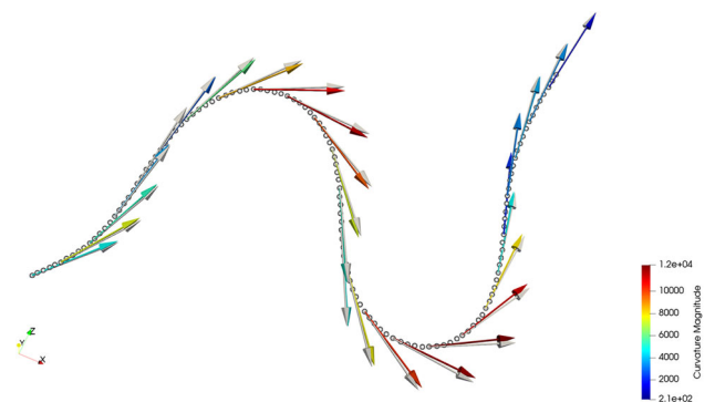
Fig. 21 Frame NO. 700 using \lambda_d = 10^{-2} , where the normal direction \mathbf{d}_3 of the cross section detaches from the tangential direction \partial_s \mathbf{x} of the centreline: \mathbf{d}_3 in white colour and \partial_s \mathbf{x} is colourful showing the magnitude of the generalised curvature. (Color figure online)
