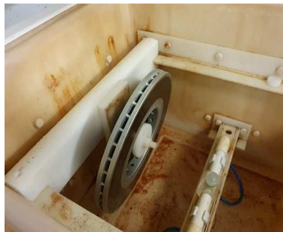
Fig. 2. Salt spray cabinet housing a brake disc
