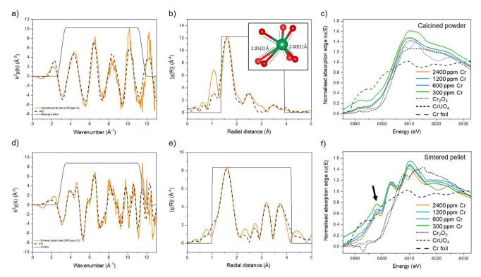
Fig. 2 Crystal structure and local coordination analysis of Cr in Cr-doped  $UO_2$  determined by EXAFS and XANES analysis.  $k^3$ -weighted Cr K-edge spectra, EXAFS model fits and Cr K-edge XANES spectra of Cr-doped  $UO_2$  in comparison to known standards ( $Cr_2O_3$ ,  $CrUO_4$  and  $Cr^0$  foil), respectively, for (**a-c**) calcined powders; and (**d-f**) sintered pellets. For (**a, b, d, e**) orange lines are data and black dashed lines are the fits.
