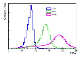
**Fig. 30** Particle identification using *PIDA* for muons and kaons in simulated proton decay events,  $p \to K^+ \overline{\nu}$ , and protons in simulated atmospheric neutrino background events. The curves are normalized by area.
