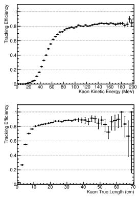
**Fig. 29** Tracking efficiency for kaons in simulated proton decay events,  $p \to K^+ \overline{\nu}$ , as a function of kaon kinetic energy (top) and true path length (bottom).
