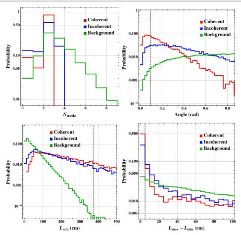
**Fig. 15** Event kinematic distributions of signal and background considered for the selection of muonic trident interactions in the ND LArTPC: number of tracks (top left), angle between the two main tracks (top right), length of the shortest track (bottom left), and the difference in length between the two main tracks (bottom right). The dashed, black vertical lines indicate the optimal cut values used in the analysis.
