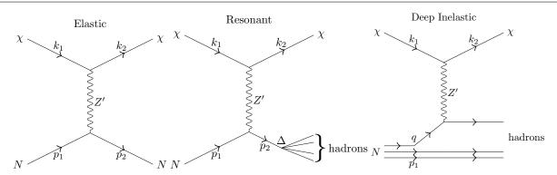
Fig. 24 Diagram illustrating each of the three processes contributing to dark matter scattering in argon: elastic (left), baryon resonance (middle), and deep inelastic (right).
