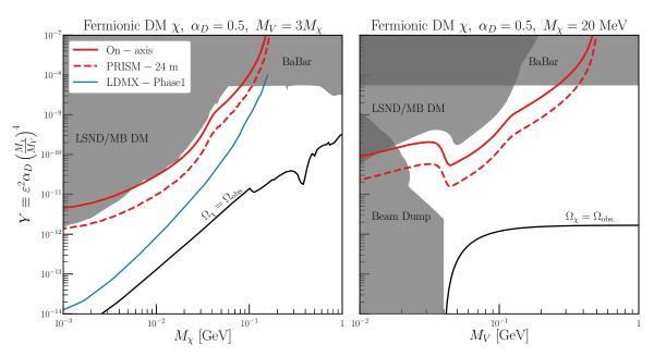
Fig. 19 Expected DUNE On-axis (solid red) and PRISM (dashed red) sensitivity using  $\chi e^- \rightarrow \chi e^-$  scattering. We assume  $\alpha_D = 0.5$  in both panels, and  $M_V = 3M_{\chi}$  ( $M_{\chi} = 20$  MeV) in the left (right) panel, respectively. Existing constraints are shown in grey, and the relic density target is shown as a black line. We also show for comparison the sensitivity curve expected for LDMX-Phase I (solid blue) [195].
