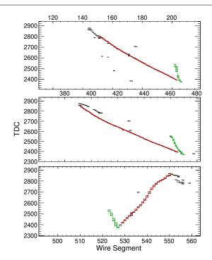
**Fig. 32** Event display for an easily recognizable  $p \to K^+ \overline{\nu}$  signal event. The vertical axis is TDC value, and the horizontal axis is wire number. The bottom view is induction plane one, the middle is induction plane two, and the top is the collection plane. Hits associated with the reconstructed muon track are shown in red, and hits associated with the reconstructed kaon track are shown in green. Hits from the decay electron can be seen at the end of the muon track.
