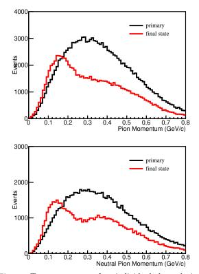
Fig. 34 Top: momentum of an individual charged pion before and after final state interactions. Bottom: momentum of an individual neutral pion before and after final state interactions.
