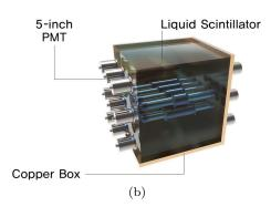
Fig. 1 Detector geometry (front view) used in the Geant4 simulation. (a) Two white-colored cylindrical shapes inside the center box represent the NaI(Tl) detectors supported by the acrylic frame (red) inside the liquid scintillator. (b) Eighteen 5-inch PMTs are attached to two sides of the copper box to detect LS-produced photons.
