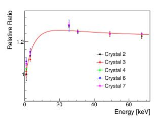
Fig. 2 Detector response to the calibration data points is described by an empirical function (red line) for five NaI(Tl) crystals at low energy.
