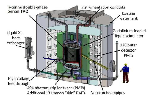
FIG. 1. Cutaway view of the LZ experiment.
