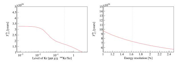
FIG. 5. Dependence of the sensitivity to the  $2\nu 2\beta$  decay of <sup>134</sup>Xe with the level of <sup>85</sup>Kr contamination in LXe (left), and dependence of the sensitivity to the  $0\nu 2\beta$  decay of <sup>134</sup>Xe with the energy resolution at Q = 825.8 keV (right). The gray dashed line indicates the values assumed in this work, namely 0.3 ppt g/g <sup>nat</sup>Kr/Xe and 1.62%, respectively.
