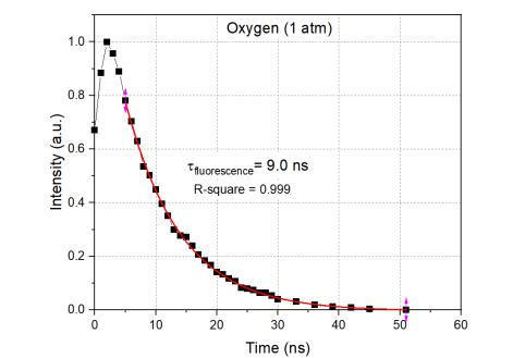
Measured fluorescence decay for  $O(3p ^3P) - 1 slm He, 0.1%H<sub>2</sub>O$
