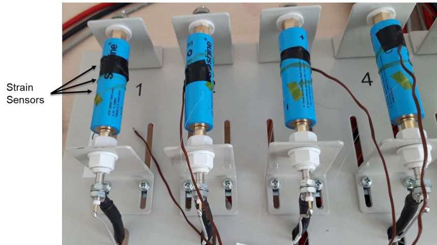
Fig. 1. Battery cycling setup, with embedded FBG-based strain sensors.
