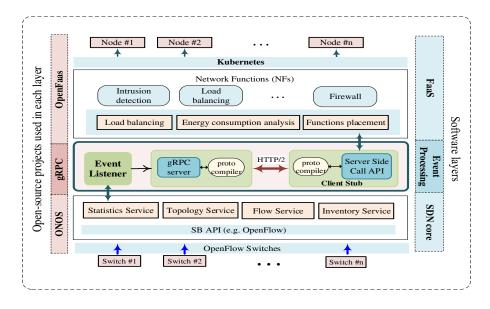
Fig. 1. A FaaS architecture for modular SDN.
