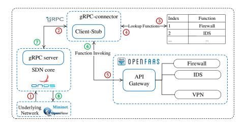
Fig. 2. ONOS and OpenFaaS Integration Sequense Diagram.
