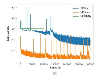
FIGURE 5 Convergence of the loss functions for (a) a weakly and (b) a strongly imposed Dirchlet boundary condition.
