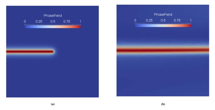
**FIGURE 10** a) Finite element ground truth b) Deep learning prediction with tanh activation function; for the prescribed displacement of  $5 \times 10^{-3}$  mm
