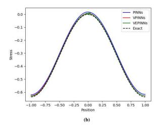
FIGURE 3 (a) Displacements and (b) stresses with a weakly imposed Dirchlet boundary condition.
