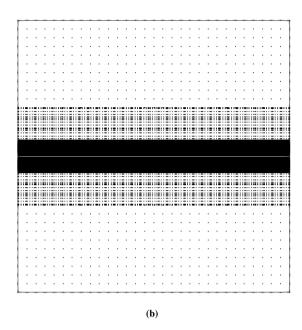
FIGURE 9 a) Geometry and boundary conditions. b) Collocation/integration points distribution
