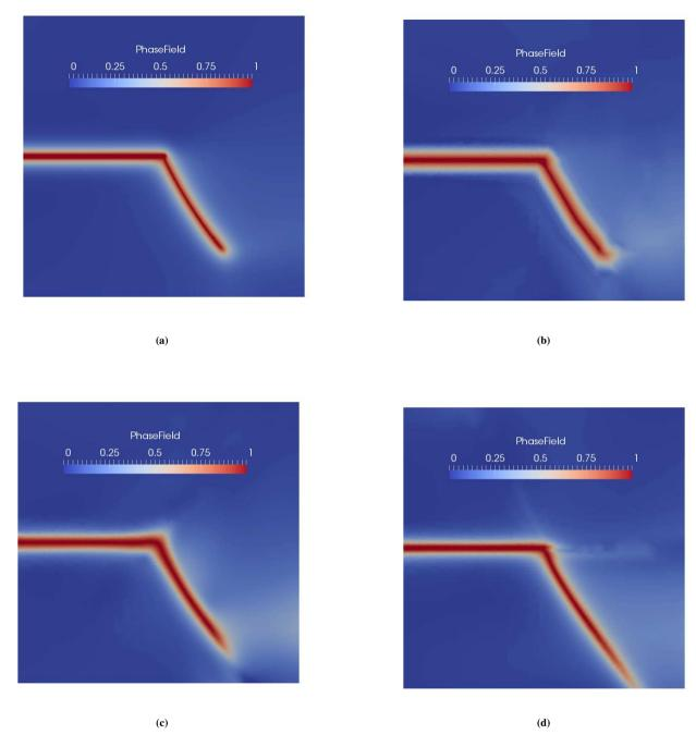
**FIGURE 14** a) Finite element ground truth b) Deep learning prediction with *ReLU* activation function c) Deep learning prediction with *softplus* activation function d) Deep learning prediction with *tanh* activation function; for the prescribed displacement of  $1.2 \times 10^{-3}$  mm.
