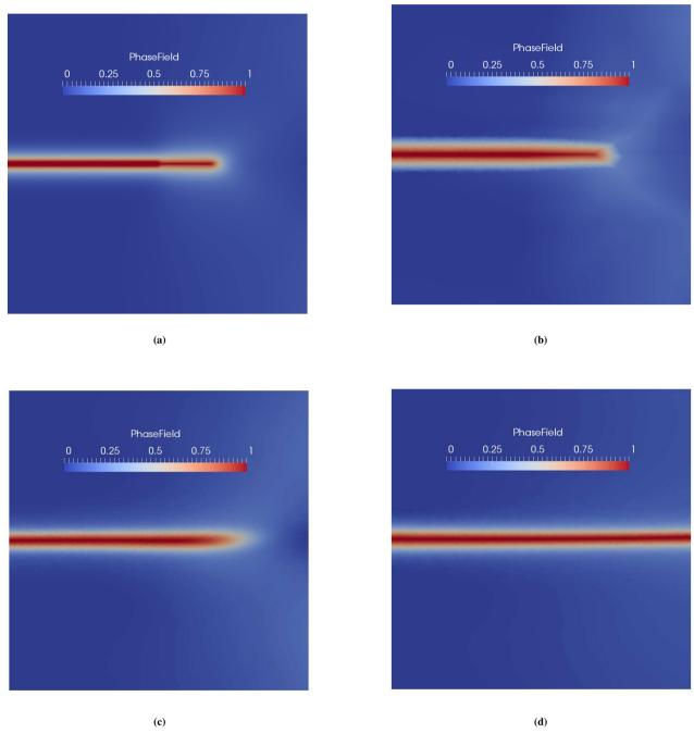
**FIGURE 11** a) Finite element ground truth b) Deep learning prediction with *ReLU* activation function c) Deep learning prediction with *softplus* activation function d) Deep learning prediction with *tanh* activation function; for the prescribed displacement of  $6 \times 10^{-3}$  mm.
