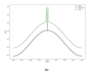
FIGURE 2 Comparison of displacements (a) and stresses (b) for solutions obtained with PINNs, isogeometric phase-field collocation method and exact solution.
