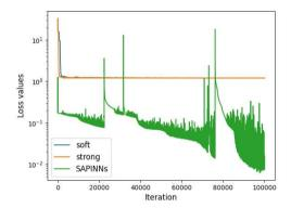
FIGURE 8 Convergence of the loss functions for soft, strong and self-adaption VE-PINNs.
