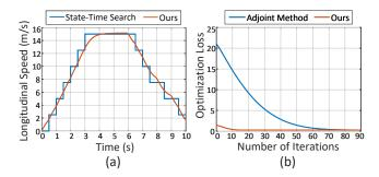
**Figure 7:** (a) The longitudinal speeds of the vehicle generated by state-time search and our method with the same keyframe constraints. (b) The optimization loss over different numbers of iterations of the adjoint method initialized with average speed and our method with the same keyframe constraints.
