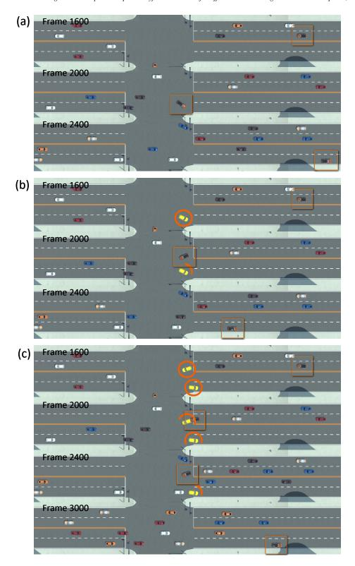
**Figure 9:** The second failure case. (a) The vehicle behaves abnormally when performing a high-speed U-turn. (b) The first solution is to assign a keyframe that causes the vehicle to simply decelerate when passing through the curve. (c) The second solution is to assign two keyframes, one to wait for oncoming vehicles and one to complete the U-turn, to further prevent aggressive driving and maintain polite behavior.
