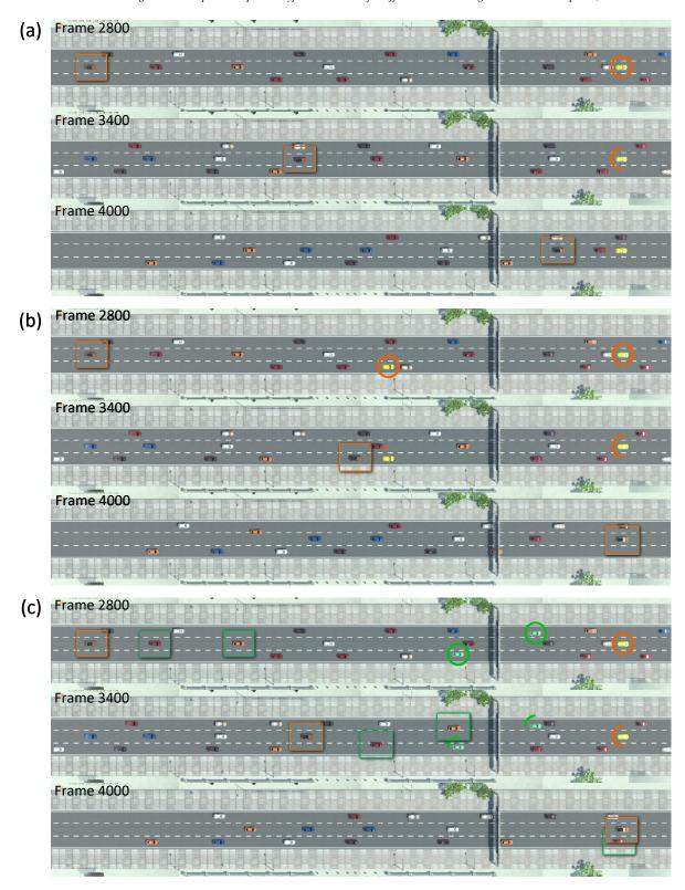
**Figure 8:** The first failure case. (a) The vehicle misses the keyframe due to traffic congestion. (b) The first solution is to give the vehicle another keyframe that causes it to overtake the leader. (c) The second solution is to assign keyframes to its leaders, forcing them to yield.
