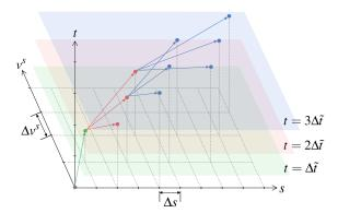
**Figure 4:** A part of discretized state-time space and directed state-time graph. The reachable nodes are marked by the dots with different colors laying on the corresponding s-v<sup>s</sup> planes, representing time at  $\Delta \tilde{t}$  (green),  $2\Delta \tilde{t}$  (red) and  $3\Delta \tilde{t}$  (blue). The transitions from parent nodes denoted by arrows are also colorized.
