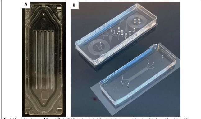
**Fig. 4** Microfluidic platforms. **A** Parsortix<sup>TM</sup> microfluidic platform for isolating circulating tumor cells based on their size and their deformability properties; **B** Image of PDMS microsystems dedicated to particle separation: spiral microfluidic systems (top); deterministic lateral displacement particle separation system (down). Both are placed on 60 × 22 mm coverslips
