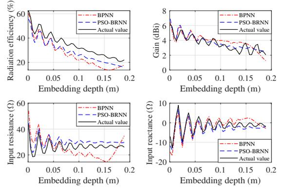
Fig. 6. Generalisation capability comparison of BPNN and PSO-BRNN
