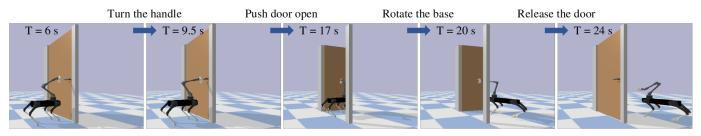
Fig. 2. Snapshots of the robot opening a spring-loaded door and walking pass.
