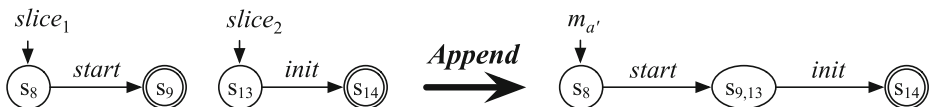
Fig. 4 Illustration of appending two sliced models generated by Slice for l_{c,1} = \langle e_{1,1} \rangle and l_{c,2} = \langle e_{2,1} \rangle . They are appended by Append , resulting in m_{a'} that accepts \langle e_{1,1}, e_{2,1} \rangle
