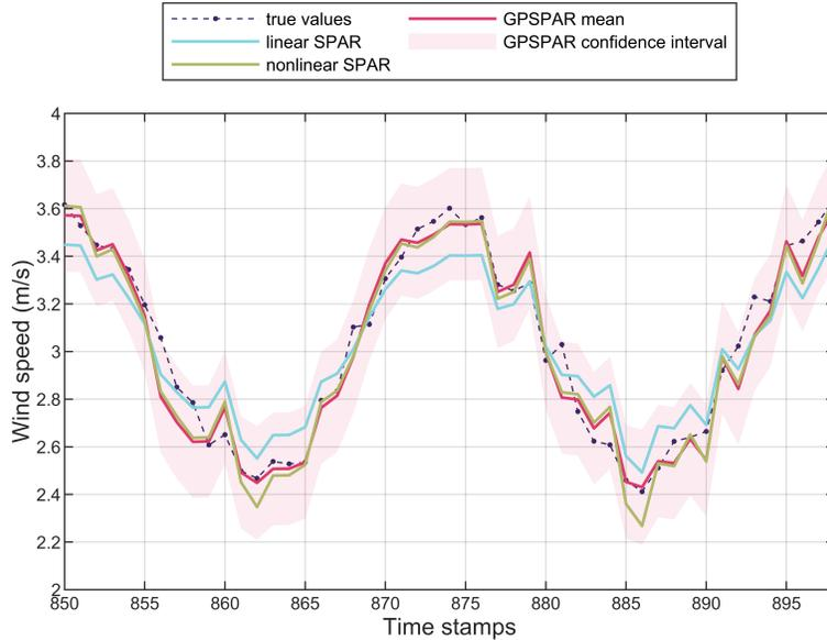
Fig. 7: Time series of wind speed predictions at turbine B3.
