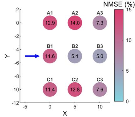
Fig. 5: NMSE of MPO predictions given by the nonlinear SPARX model.
