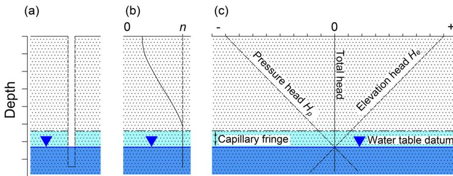
**FIGURE 3** The water table in an idealized porous medium or classical soil. (a) Well (see Section 4.2) showing the position of the water table, below a saturated capillary fringe. (b,c) Soil water content and soil-water energy status vertically above and below the water table.  $N$  denotes (total) porosity. Based on original figures in Price (1996) and Freeze and Cherry (1979).
