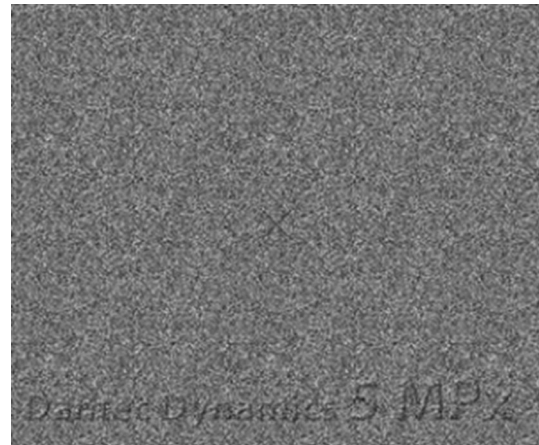
Fig. 4 5MP speckle pattern
