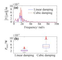
**Fig. 7** The output responses and energy harvesting performance of system (27) subject to input 2 under linear and cubic damping
