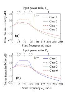
Fig. 4 The power transmissibility against the range of input frequencies (represented by  $\omega_{st}$ )/power ratio of input  $\Upsilon_{in}$
