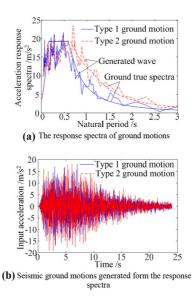
Fig. 11 The response spectra and corresponding time history of seismic ground motions
