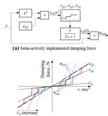
(b) Semi-active damping forces under different control laws
