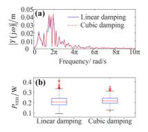
Fig. 6 The output responses and energy harvesting performance of system (27) subject to input 1 under linear and cubic damping
