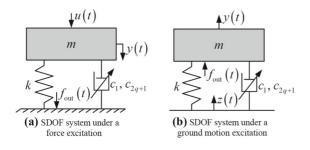
Fig. 1 SDOF systems with antisymmetric nonlinear damping
