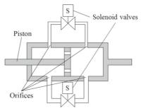
Fig. 9 The structure of the semi-active damper
