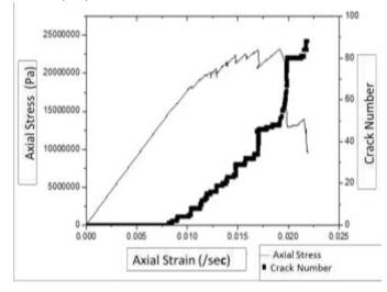
Fig. 5. Strain data and Corresponding crack number for  $(x10^{4})$  particle used for simulation
