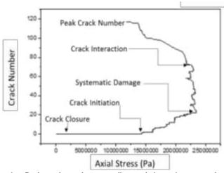
Fig. 6. Crack number and corresponding crack interaction stages: the mechanism of micro-fracturing of Ughelli sandstone at 5 stages for  $(x10^{4})$  particles used for simulation
