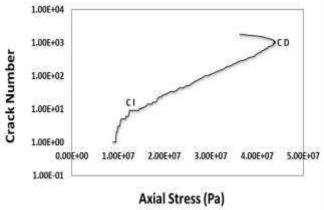
Fig. 3. Crack Initiation (CI) and crack damage (CD) stresses for unconfined axial stress application. The crack number are limited to  $(1x10^{4})$  particles used for building sandstone sample in the Discrete Element Modelling (DEM).
