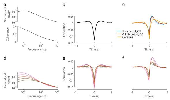
**Fig. 3** Simulation of the effect of amplifier high-pass filter on measured cross-correlations. **a** The power spectrum and coherence of a synthetically generated pair of signals x(t) and y(t) (see Methods). **b** The symmetric cross-correlation between x(t) and y(t). **c** The cross-correlation after y(t) was filtered with the amplifier transfer functions shown in Fig. 2c-d. **d** Pairs of synthetic signals x(t), y(t) were generated
