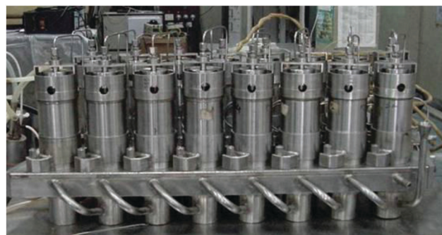
Fig. 22 CORAL 16-stage 35 mm CC cascade.
