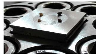
Figure 4 Sand Placement on HPT Sample.
