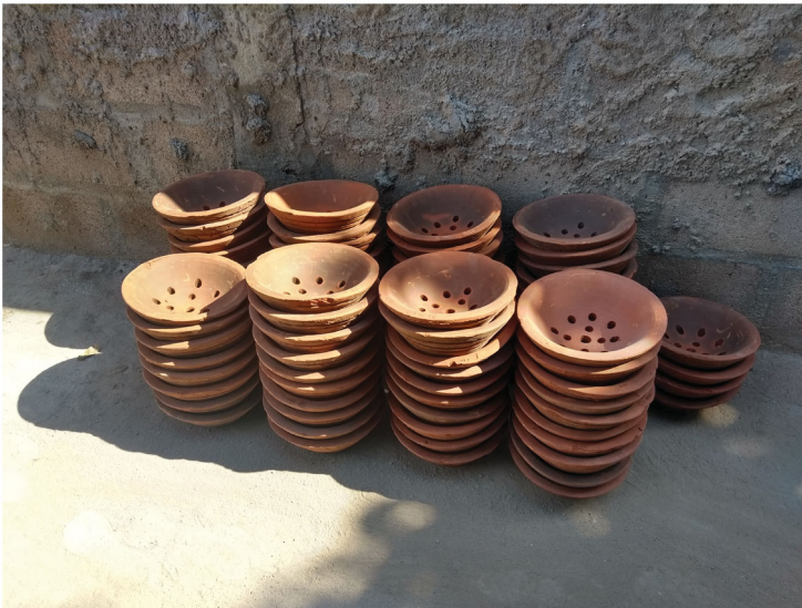
Figure 4. Ceramic liners that make use of local skills.
