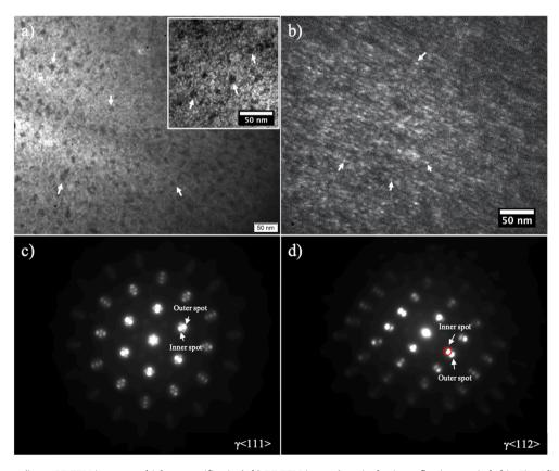
Fig. 6. a) BF-TEM image (inset: BF-TEM image at a higher magnification), b) DF-TEM image (acquired using reflections encircled in Fig. 6d), and c) corresponding EDPs for the topmost treatment layer (taken at depth  $< 1 \mu m$ ) on alloy 718 after TPN treatment at 450 °C for 20 h.
