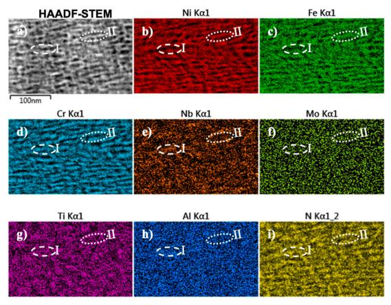
Fig. 8. STEM-EDX analysis for the topmost surface (images taken at depth  $< 1 \mu m$ ) on 700-1, a) HAADF-STEM image, b) corresponding EDX maps for b) Ni, c) Fe, d) Cr, e) Nb, f) Mo, g) Ti, h) Al, and i) N. Two regions were highlighted by circles to guide viewing. Note that element maps in Fig. 8b-i do not perfectly superimpose with Fig. 8a owing to sample drift during prolonged EDX elemental scan.
