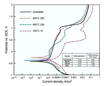
Fig. 11. Potentiodynamic polarization curves for alloy 718 before and after TPN treatment at 400  $^{\circ}$ C for 20 h, at 450  $^{\circ}$ C for 20 h and at 700  $^{\circ}$ C for 1 h.
