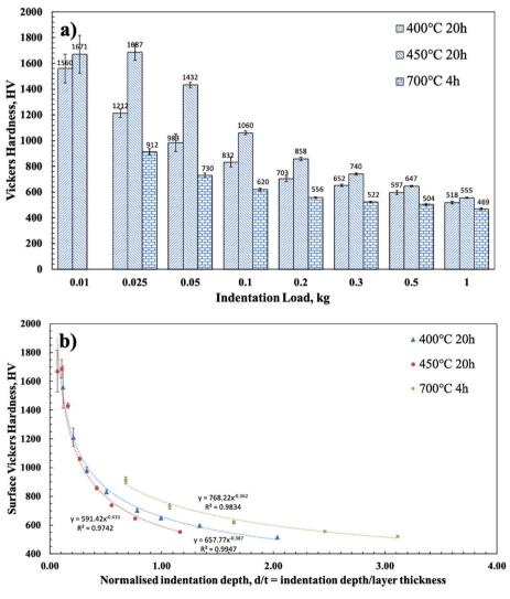
Fig. 10. Surface Vickers hardness of alloy 718 after TPN treatment at  $400 \,^{\circ}$ C for 20 h, at  $450 \,^{\circ}$ C for 20 h and at  $700 \,^{\circ}$ C for 4 h under different indentation loads (i.e. 0.01, 0.025, 0.05, 0.1, 0.2, 0.3, 0.5 and 1 kg). a) bar chart for hardness against indentation load and b) plot for the measured hardness value against normalised indentation depth (d/t = indentation depth/layer thickness).
