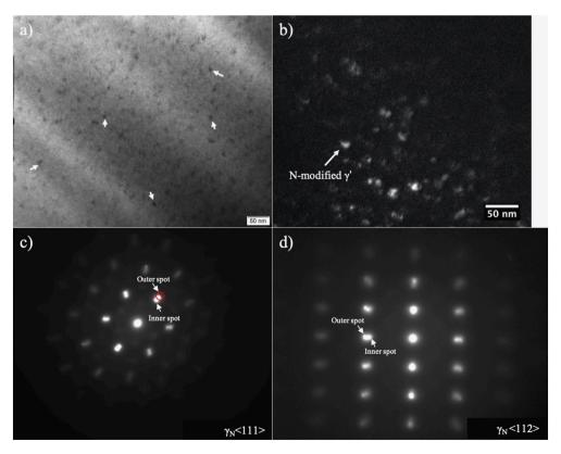
Fig. 5. a) BF-TEM image, b) DF-TEM image (acquired using reflections encircled in Fig. 5c), and c, d) corresponding EDPs for the treatment layer (taken at depth < 1  $\mu$ m) on alloy 718 after TPN treatment at 400 °C for 20 h.
