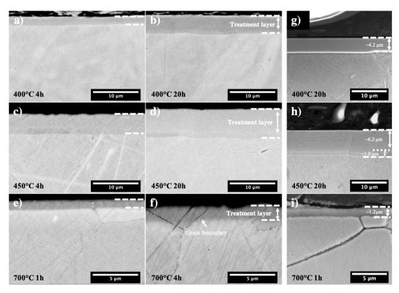
Fig. 2. BS-SEM images for Inconel 718 cross-sections (without etching) after TPN treatment at a) 400 °C for 4 h, b) 400 °C for 20 h, c) 450 °C for 4 h, d) 450 °C for 20 h, e) 700 °C for 1 h, and f) at 700 °C for 4 h; and SEM images for Inconel 718 cross-sections (after etching) after TPN treatment at g) 400 °C for 20 h, h) 450 °C for 20 h, and i) 700 °C for 1 h. Note the scale bar is 5  $\mu$ m in Fig. 2e & f & i.
