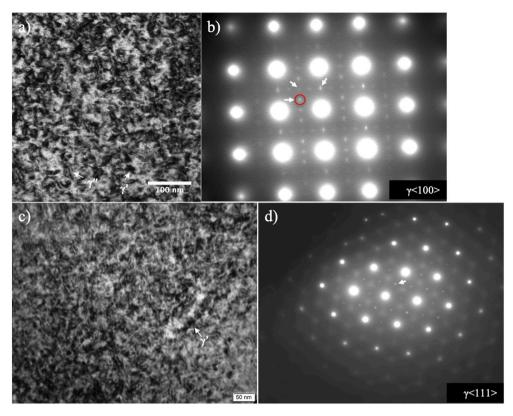
Fig. 4. BF-TEM images and corresponding EDPs for the unmodified core of alloy 718 treated at a, b) 700 °C for 1 h and c, d) at 400 °C for 20 h, showing  $\gamma'/\gamma''$  nanoprecipitation morphology. Superlattice reflections are indicated by arrows in Fig. 4b & d.
