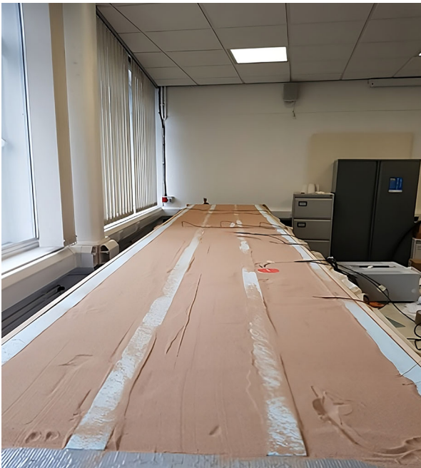
Fig. 6. A photograph of the buried pipe system in the sand.
