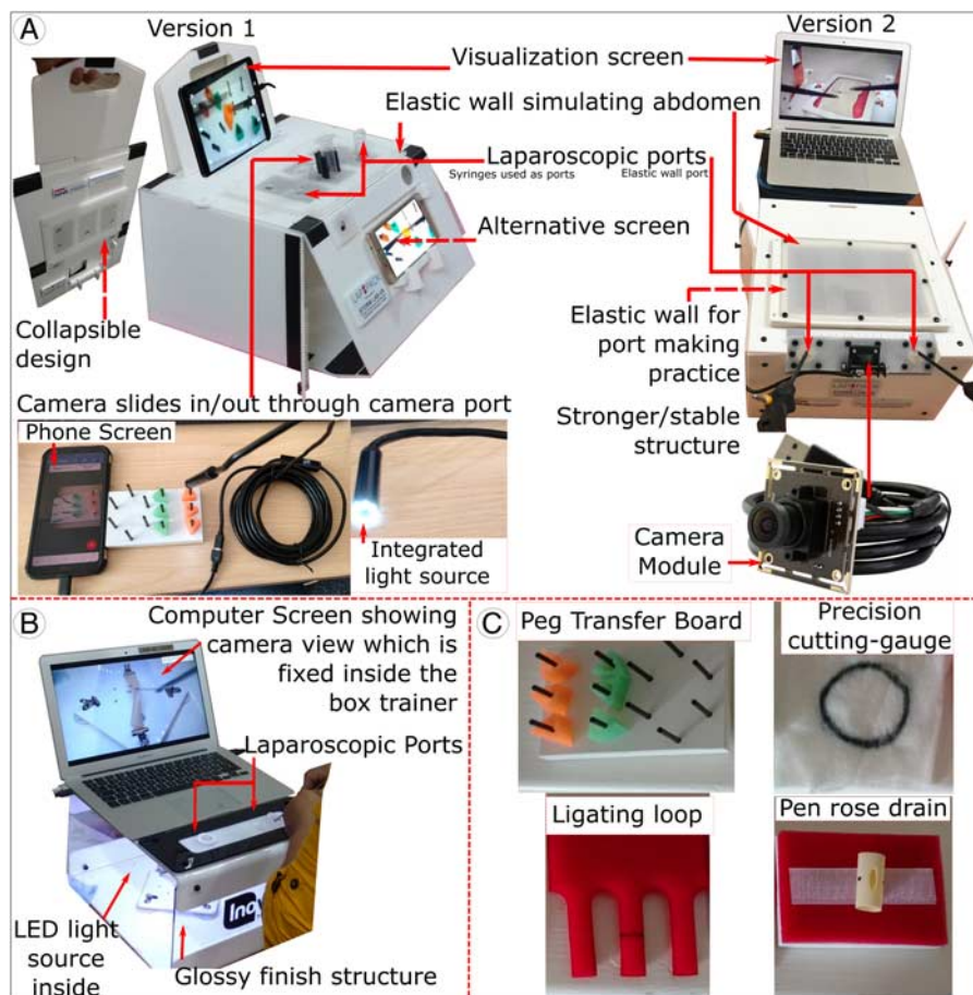
Figure 1. Design features of Lap-Pack; (A) version 1 and version 2. B, Design features of Inovus box trainer. C, Consumable task for laparoscopic training.
