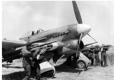
Armourers fit rocket-projectiles to the under-wing racks of a 247 Squadron Hawker Typhoon IB at B6/Coulombs, Normandy, on 16 June 1944.
