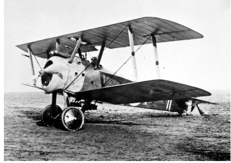
Sopwith Camel of 46 Squadron fitted with four 25lb Cooper bombs under the fuselage, 16 December 1917. It has a flight commander's pennant fitted to the rudder.
