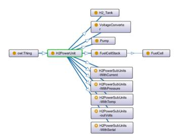
Fig. 6. Asserted ontology for hydrogen car power unit.
