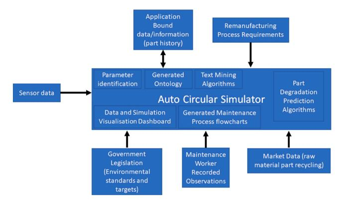
Fig. 9. Schematic of the Auto Circular Simulator and data/information flows.
