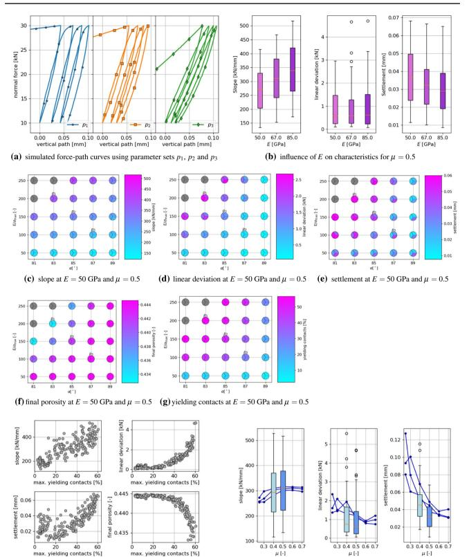
(h) correlations of slope, linear deviation, settlement and percentage of yielding contacts for simulations using  $\mu = 0.5$
