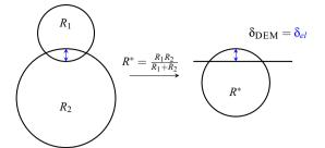
(a) purely elastic case: real contact configuration (left) and imagined equivalent sphere-plane contact (right)
