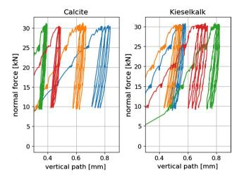
Fig. 2 Examples of compression tests for the two types of ballast. Different colours correspond to repetitions of the same test
