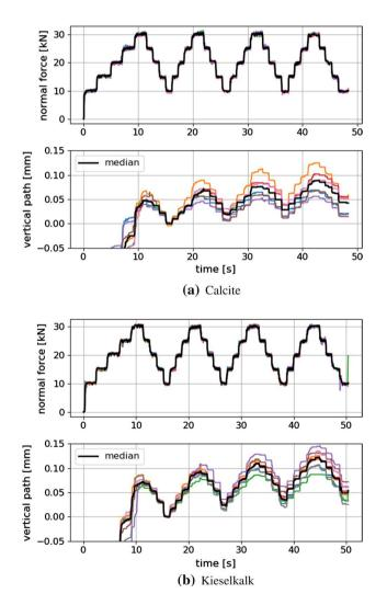
Fig. 3 Time-warped path and force signals plotted over time, single measurements and median curve, for both types of ballast
