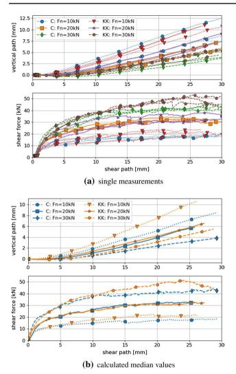
**Fig. 5** Shear force and vertical path plotted over shear path for Calcite (C) and Kieselkalk (KK)
