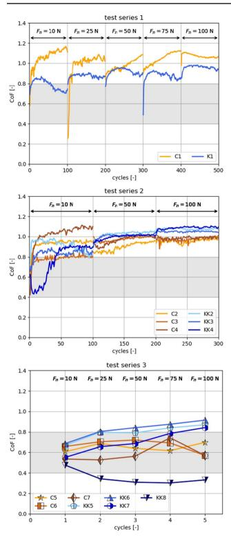
**Fig. 6** CoF plotted over cycles for both Calcite (C) and Kieselkalk (KK) for test series 1, 2 and 3. The grey shaded areas correspond to values of the CoF typically used in DEM simulations of railway ballast in the literature
