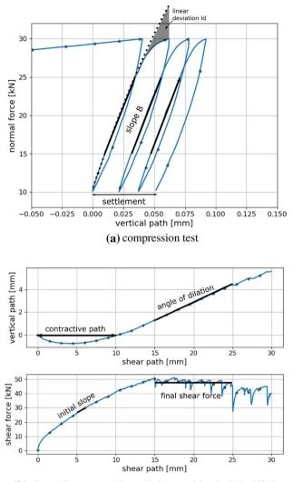
(b) direct shear test with applied normal load of  $F_n=10$ kN
