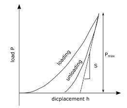
Fig. 7 Sketch of load displacement curve for an indentation experiment, redrawn from [26]
