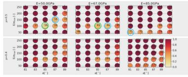
(c)  $\varepsilon$  over parameter space using  $\hat{p}_2$ : E = 55 GPa,  $E/\sigma_{max} = 102, \alpha = 85.5^\circ, \mu = 0.52$
