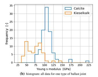
Fig.8 Measured values of Young's modulus for Calcite and Kieselkalk
