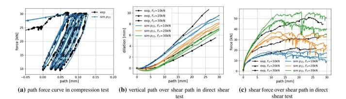
Fig. 19 Experimental results plotted together with simulation results of  $p_{23}$ : E = 50GPa,  $E/\sigma_{max} = 100, \alpha = 82^\circ, \mu = 0.45$
