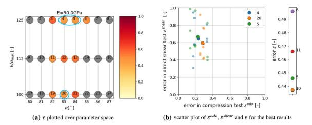
Fig. 22 Parametrisation for shape no. 9, step 3: refined parameter space, simulations with three initial configurations
