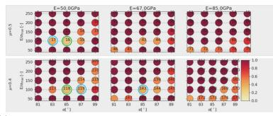
(a)  $\varepsilon$  over parameter space using  $\hat{p}_5$ : E = 51 GPa,  $E/\sigma_{max} = 102, \alpha = 85.5^\circ, \mu = 0.44$
