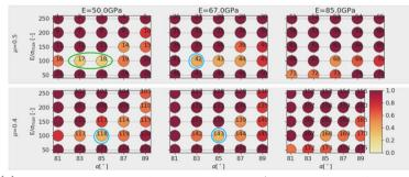
(g)  $\varepsilon$  over parameter space using  $\hat{p}_4$ : E = 51 GPa,  $E/\sigma_{max} = 102, \alpha = 84^\circ, \mu = 0.52$  (h)  $\hat{p}_4$ :  $\varepsilon^{odo}, \varepsilon^{shear}$  (left plot) and  $\varepsilon$  (right plot)
