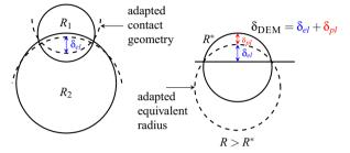
(b) damage / plastic yielding: real contact configuration (left) and imagined equivalent sphere-plane contact (right)
