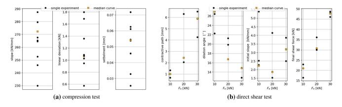
Fig. 14 Evaluations of experimental data of Kieselkalk ballast w.r.t. characteristics for compression and direct shear test characteristics. Plotted are the characteristics of the single experiments and the characteristics of the median curve calculated in Sect. 2.1
