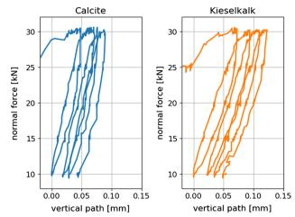
Fig. 4 Median curves of normal force and vertical path of compression tests for both Calcite and Kieselkalk
