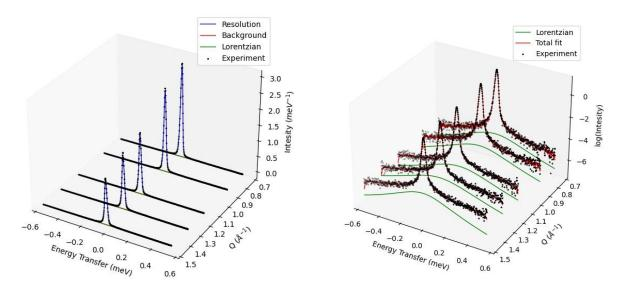
**Figure S11.7.** Subtracted QENS spectra of 7.34 wt% methanol loaded commercial FER at 273K at Q = 0.74, 0.91, 1.16, 1.33, and 1.49  $\text{Å}^{-1}$ . Left hand plot shows raw intensity, right hand shows log intensity. Selected spectra shown for clarity.
