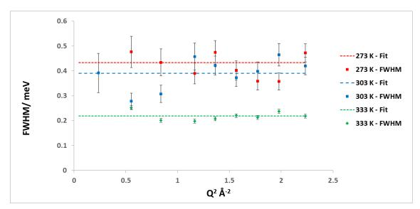
**Figure SI1.9.2.** Q<sup>2</sup>-dependence of the FWHM of the Lorentzian component for the 10.18 wt% methanol loaded FER-GHA sample at 273 K, 303 K and 333 K. The dotted lines indicate a line of best fit.
