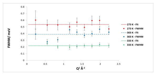
**Figure SI1.9.1.** Q²-dependence of the FWHM of the Lorentzian component for the 7.34 wt% methanol loaded commercial FER sample at 273 K, 303 K and 333 K. The dotted lines indicate a line of best fit.
