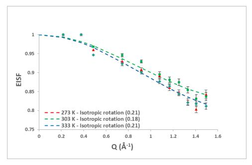
**Figure S11.8.** Experimental EISF plots for methanol in the 7.34 wt% methanol loaded commercial at 273 K, 303 K and 333 K as well as the fit of the isotropic rotation model with their commensurate mobile fractions.
