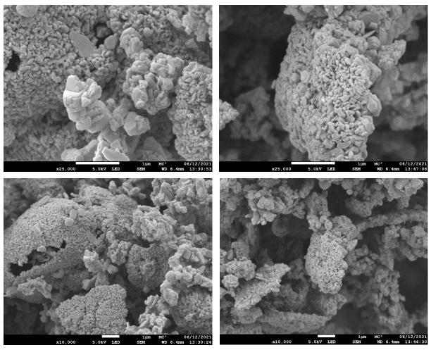
Figure SI1.4.3 SEM images of the commercial FER sample.
