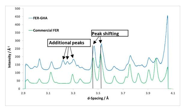
Figure SI1.5.1. Neutron diffraction patterns of Commercial and FER-GHA samples.
