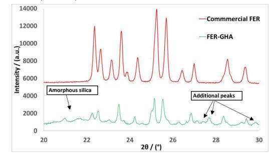
**Figure 1.5.3.** X-ray diffraction patterns of commercial FER and FER-GHA. Only 20-30° 20 is shown. Commercial FER pattern is offset by 5000 a.u. for clarity. Annotations included for detail.
