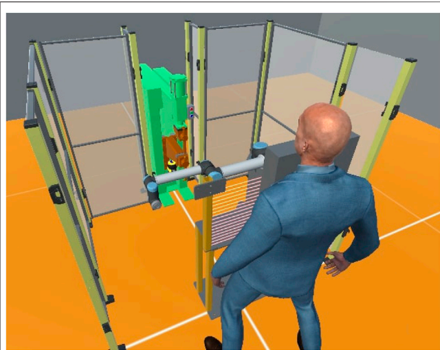
FIGURE 1 | An isometric view of the CSI framework environment applied to a collaborative welding cell case-study. Based in Unity ® 3D, digital twins of an operator, collaborative robot manipulator, safety scanner and light-barrier are shown.
