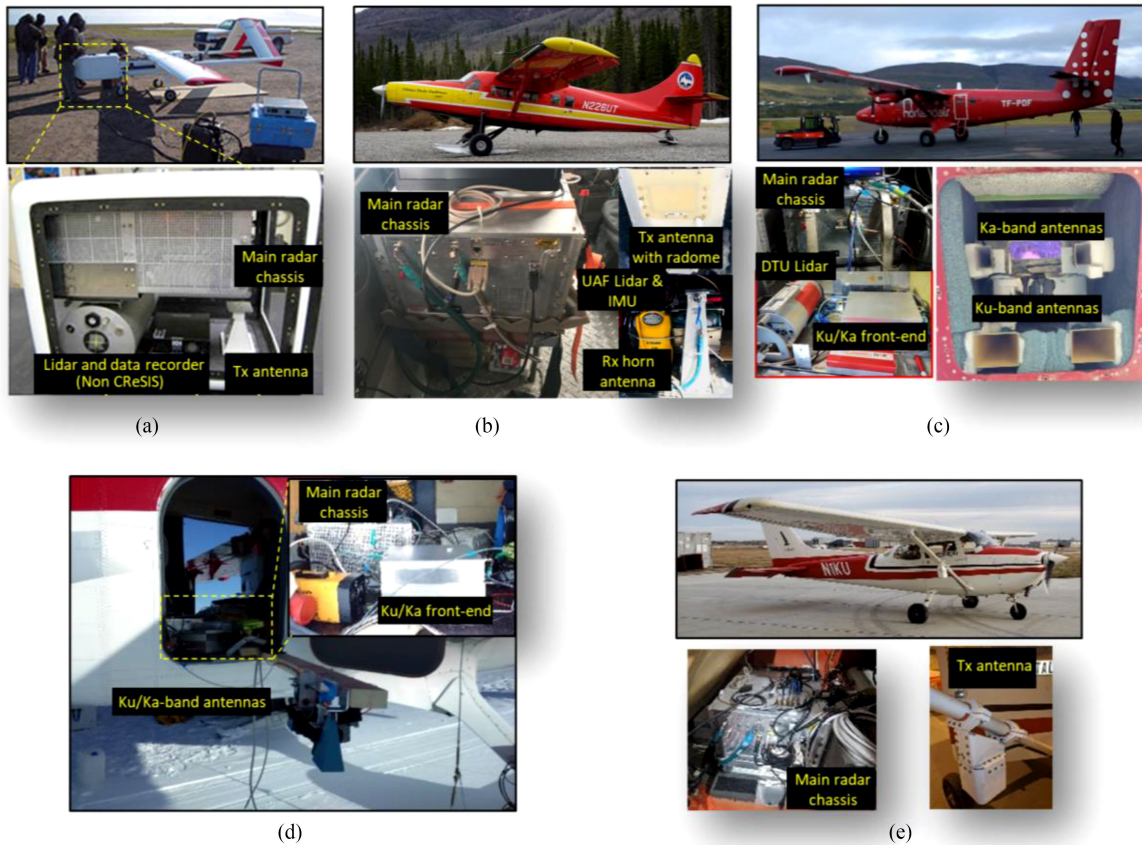
Fig. 3. Photographs showing the instrument and antenna configurations for different test platforms. (a) Integration on the NASA SIERRA UAS (not flown). (b) Integration on a de Havilland DCH-3 Single Otter for S/C band field trials in Alaska. (c) Integration on a de Havilland DHC-6 Twin Otter for Ku -/ Ka -band field trials in Greenland and Arctic sea ice. (d) Surface-based test setup for firn measurements on the Greenland Ice Sheet. (e) Instrument configuration on a Cessna 172 for S/C band trials to measure terrestrial snow cover in South Dakota.
