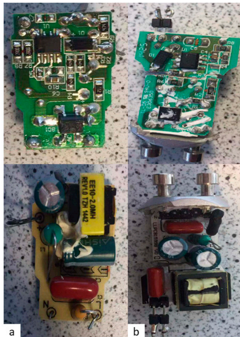
Figure 3. The two sides of both drive circuits after disassembly. Circuit boards of sample A on the left (a) and sample B on the right (b); top row: sides with tracks and ICs, bottom row: sides with discrete electrical components.
