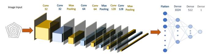
Fig. 3 CNN architecture with a pentagon image as input (left), the convolutional and max-pooling layers (middle) and the schematic representation of the feature reduction that occurs from the flattened to the output layer (right)
