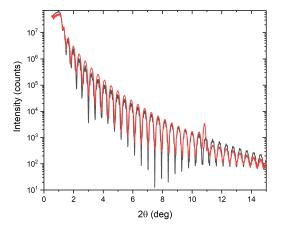
Figure 1: X-ray reflectivity data of a platinum  $C_{60}$  bilayer (red) and GenX fit (black). The structural  $C_{60}$  peak at 11° is not captured by the low angle fit.
