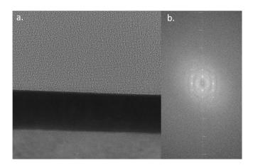
Figure 2: a. TEM obtained from the Pt/C60 bilayer lamella, showing clear molecular layers and an atomically sharp interface. b. FFT of the  $C_{60}$  layer, showing 3D crystal structure.
