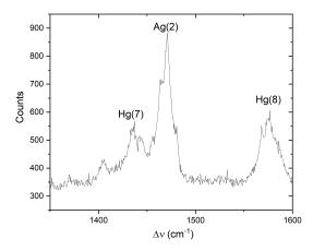
Figure 3: Raman spectrum of C<sub>60</sub> film. The three major Raman active modes are present and the characteristic mode of graphite at 1600 cm<sup>-1</sup> is absent. The splitting of the Ag(2) peak is characteristic of electron transfer across a metallic interface.
