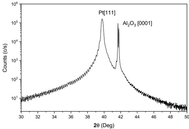
Figure 2: Out of plane X-ray diffraction data of a platinum thin film grown in the organics evaporation chamber. The Pt (111) and Al<sub>2</sub>O<sub>3</sub>(0001) Bragg diffraction peaks can be observed, in addition to Pendellosung fringes implying very smooth and flat film surfaces. The out of plane grain size measured for this film was  $43 \pm 0.4$  nm.
