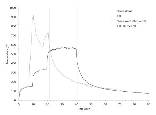
Figure 8. Volume-weighted average temperature of upper layer—burner only experiments.
