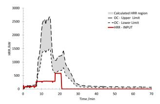
Figure 4. PIR panels—heat input and output from experiments with burner only. OC refers to measurements based on oxygen consumption calorimetry. HRR—INPUT refers to the heat release rate from the gas burner.
