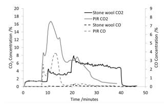
Figure 9.  ${\rm CO_2}$  and  ${\rm CO}$  concentrations at doorway—burner only experiments.
